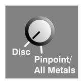
The Excalibur II can operate in two different modes. This control selects either Disc (Discriminate) or Pinpoint/All Metals mode.
